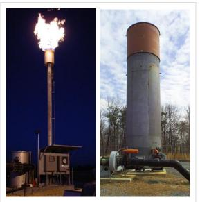
Figure 3-4. Open Flare (left) and Enclosed Flare (right)
