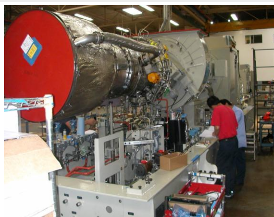
Figure 4-7: Dual Gas Wide Wobbe Fuel Assembly and Fuel Injectors on a Solar LFG Turbine 13
