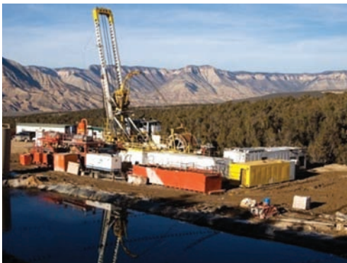
Large Hybrid Rig in San Juan Basin of Colorado, USA. Rig can effectively use conventional drill pipe or coiled tubing
