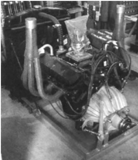
Exhibit 1. Engine Drive for Single Generator
