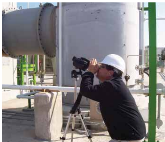
Utilizing infrared cameras to detect leaks at a natural gas facility in Mexico.
