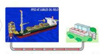
Associated gas is recovered offshore, and transported via a dense phase pipeline to a new gas separation plant, where it is processed into useful energy products and delivered to the domestic market for productive use as energy products.
