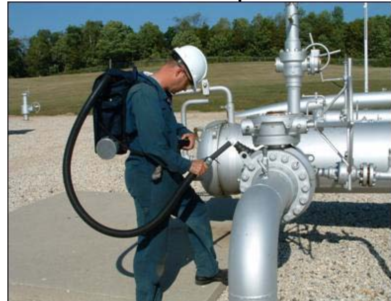
Leak Measurement Using High Volume Sampler
