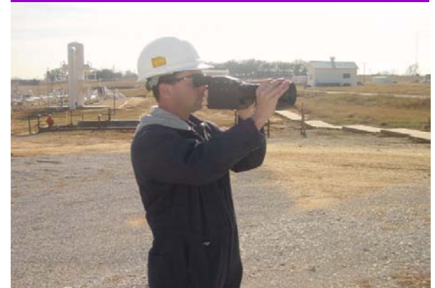
Infrared Leak Detection
