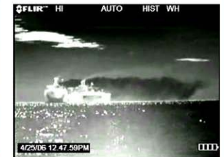
VOC emissions visible during lightering operations.
