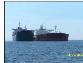
Crude oil tankers performing lightering operations.
