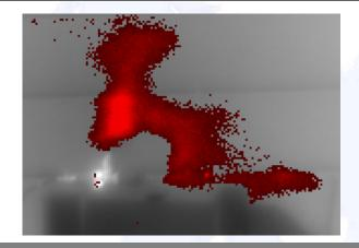
Shown above is an Ethane leak where the gas is colored red with the higher concentration shown in the brighter red. The concentration of any pixel within the gas cloud is shown on the right
