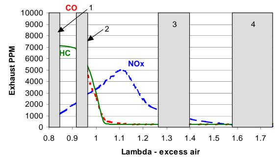
In stoichiometric or rich burn engines, much of the energy goes "up the stack" or to the catalytic converter in the form of CO and unburned methane
