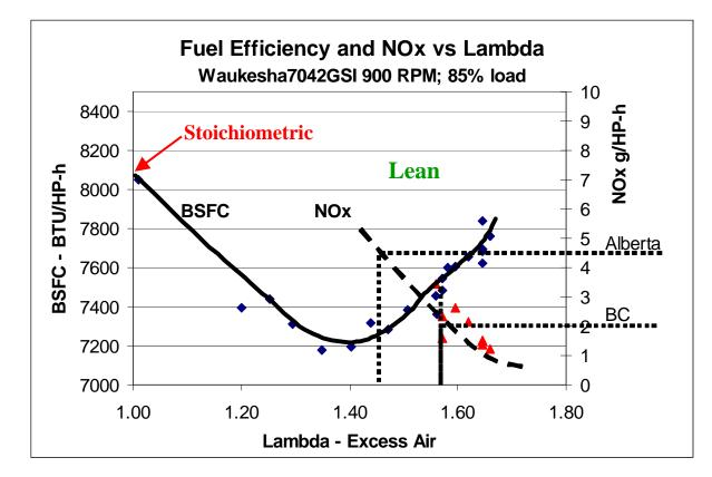
With current Alberta NOx regulations the fuel efficiency is near optimum
