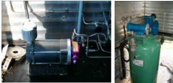
Electricity is then used to power electrical equipment or pneumatic equipment via an air compressor Solar, pressure and wind energy are captured and converted into electricity, which is stored in a bank of batteries.
