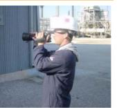
Infrared Leak Imaging Camera
