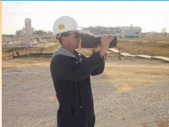
Optical Leak Imaging
