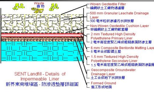
SENT Landfill - Details of Impermeable Liner
