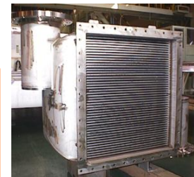
600kW-class Re-generative cycle GT : S7A
