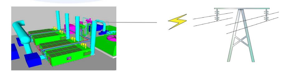
0.2 % methane needed to maintain oxidation. Energy of concentrations above 0.2 % can be recovered.
