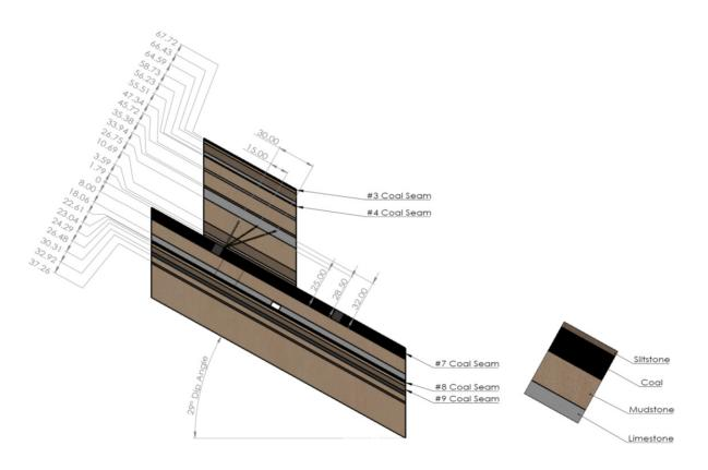
Figure 3-4: Horizontal Gob Boreholes Drilled from Mining Level (Profile View)
