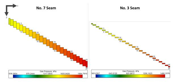
Figure 3-6: Example Model Layout for In-Seam Pre-Drainage Boreholes (Profile View)
