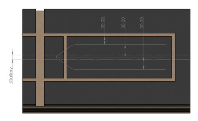
Figure 3-1: Horizontal Trunkline Boreholes Drilled from Underlying Gallery with Branchline Boreholes
