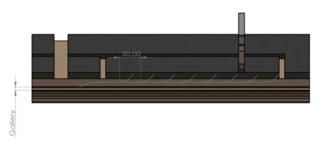
Figure 3-2: Horizontal Trunkline Boreholes Drilled from Underlying Gallery with Branchline Boreholes Drilled Upwards into Coal Seam (Profile View)
