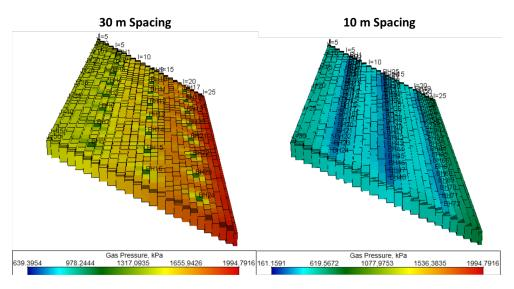
Figure 3-7: Example Model Layout for In-Seam Pre-Drainage Boreholes (3D View)
