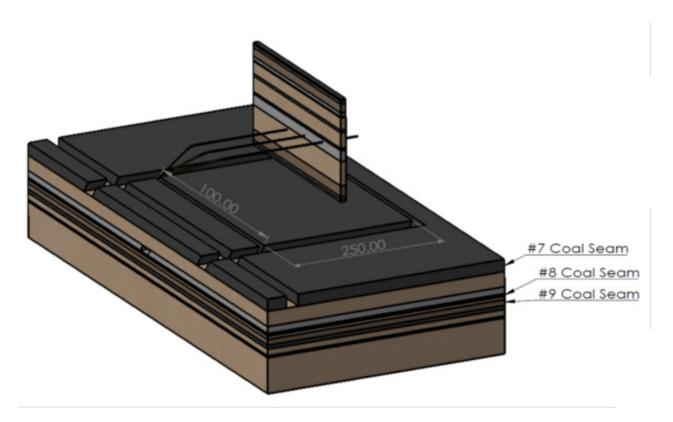
Figure 3-3: Horizontal Gob Boreholes Drilled from Mining Level
