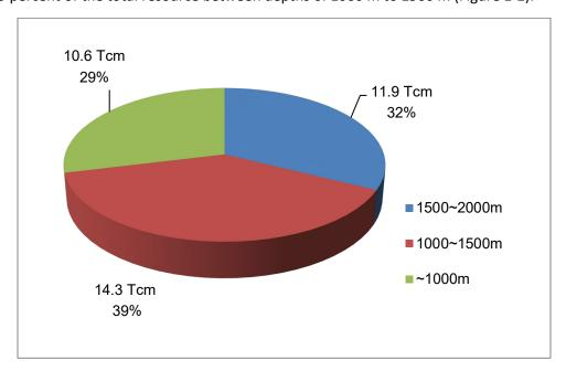
Figure 1-2: Depth of Coalbed Methane Resources in China
