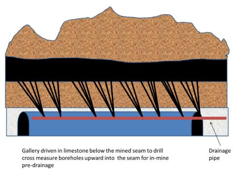
Figure 2-3: Cross-Measure Boreholes Drilled from a Gallery below the Mined Seam
