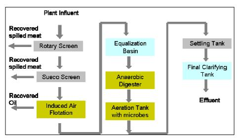
Figure 3.16 – Waste Treatment Process Flow of a DCN Plant
