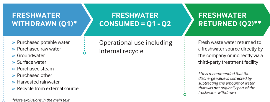
Figure 4.1: Calculation of freshwater consumption
