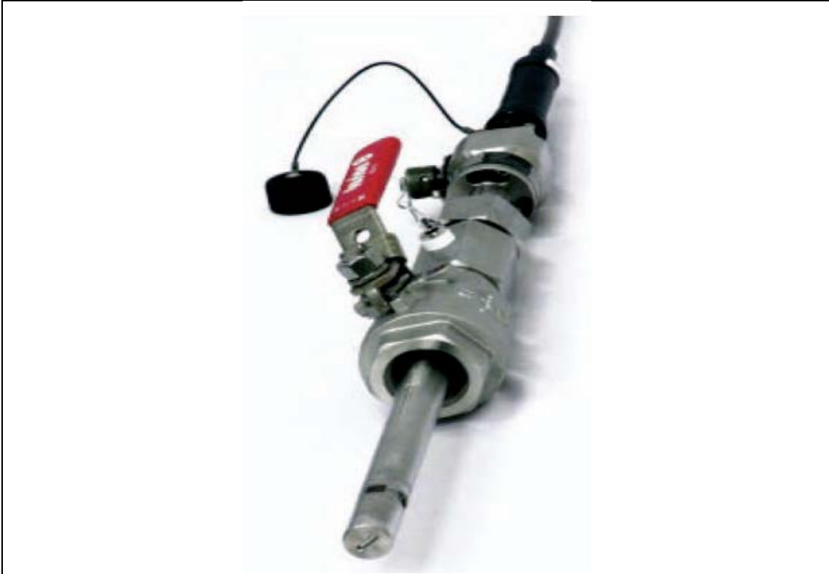
Figure 6: Photograph of an optical flow meter probe.
