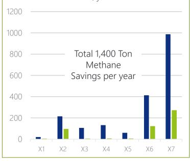
Methane Emission Reduction Results in one-year, average figures per Gas Asset type, 400 LDAR campaigns,10mio measurements. From 1,42kg/year/source to 0,92kg/year/source or -35% Average mass leak kg/year for typical source types in Gas Assets, 400 LDAR campaigns. Average improvement: from 181kg/year to 127kg/year for a leak Benchmark Campaign results for 7 gas processing plants. Total 1 400 Ton Methane emission saving per year with a one-year campaign or-70%
