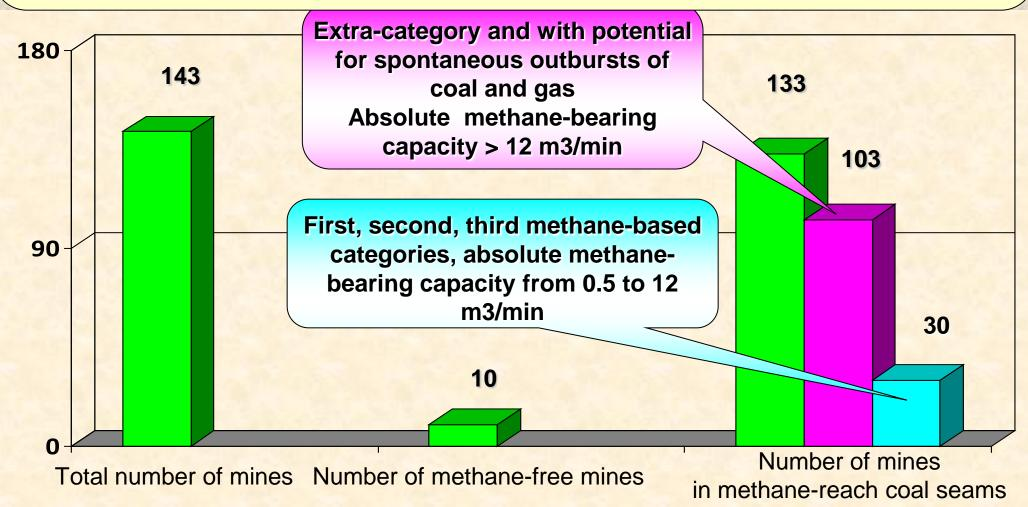
Volume of methane emissions from mines is about 1400 million m3/year. Coal production process is accompanied by natural methane gas emissions into mine ventilation system in approximate amount of 1000 million m3/year.
